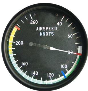
Figure 27. Airspeed indicator of a Part 23 airplane with red V_{MCA} and blue V_{YSE} lines.
