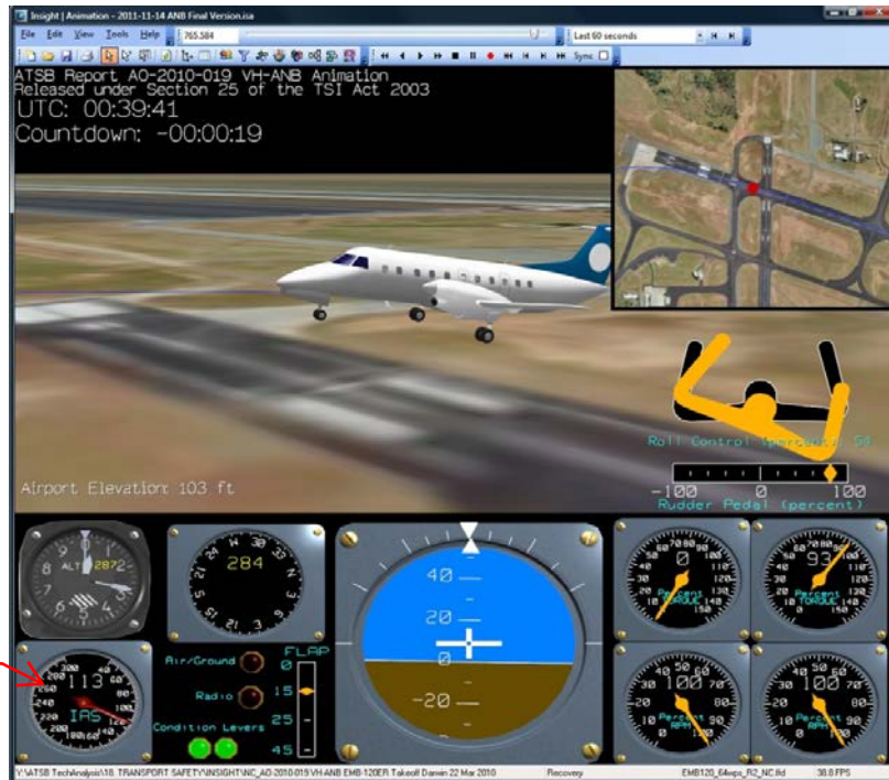
Figure C-4: Heading 20° left of runway, banking left and 8 seconds to the end of recording
