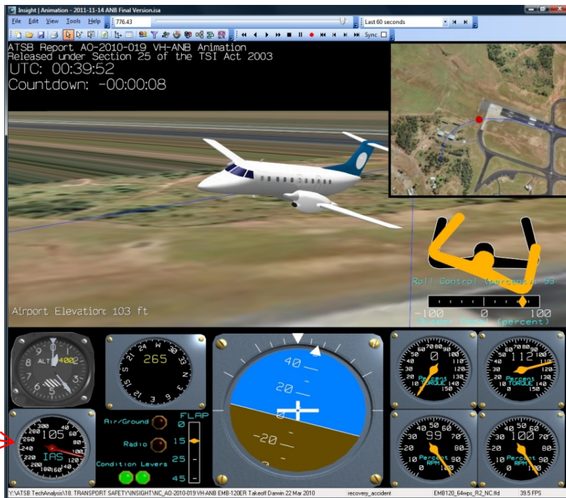
Figure C-4: Heading 20° left of runway, banking left and 8 seconds to the end of recording
