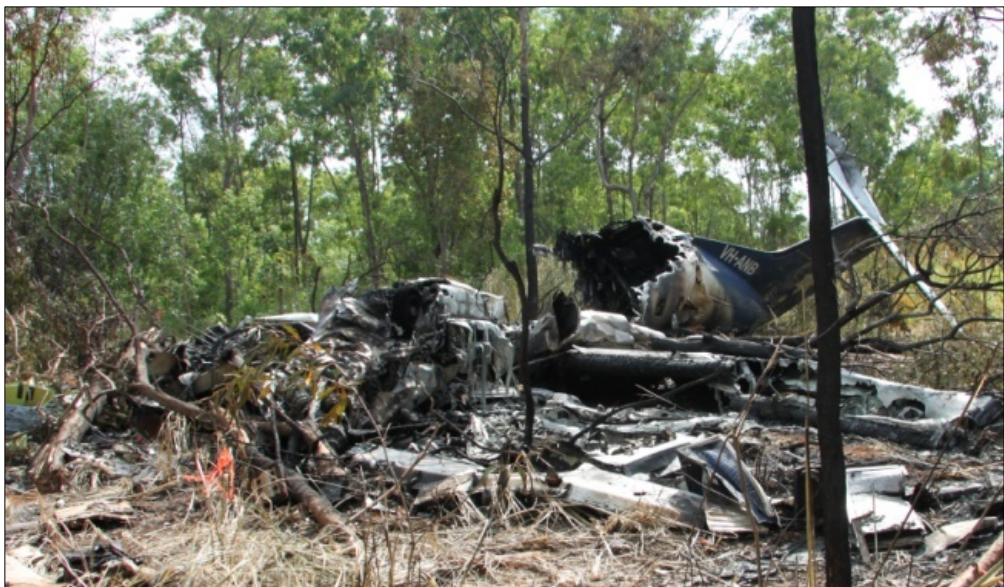
Figure 12: Aircraft wreckage, showing the extensive fire damage
