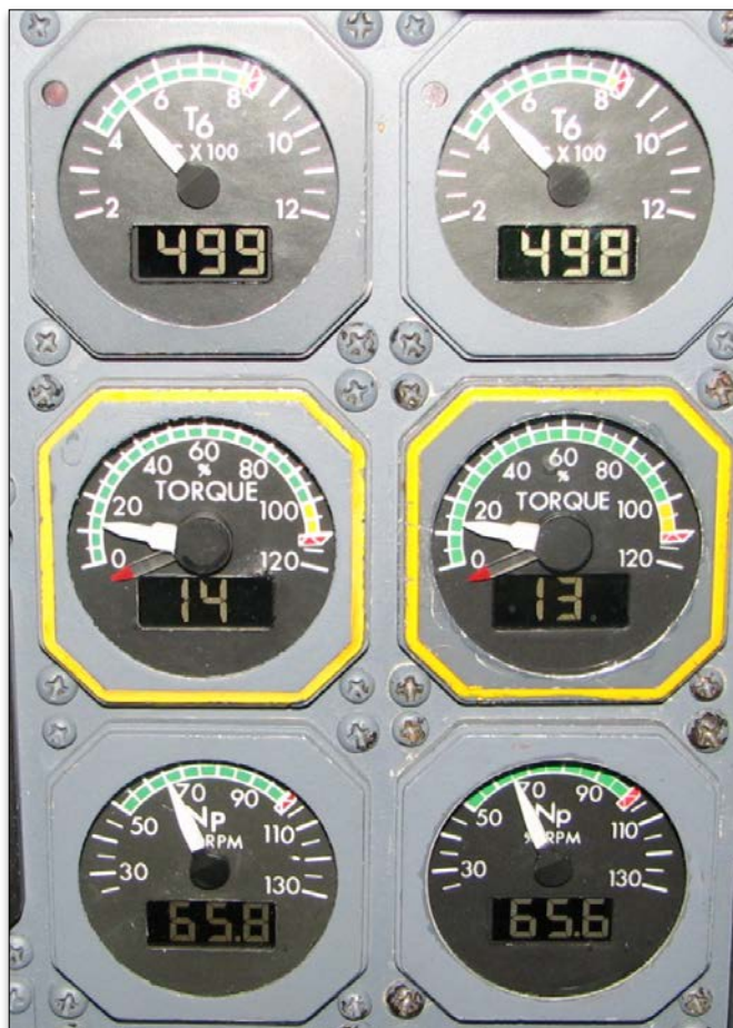
Figure 5: Engine Inter-turbine Temperature ( T_6 ) (top row) and Torque (centre row) gauges and Propeller RPM ( N_p ) gauges (bottom row)
