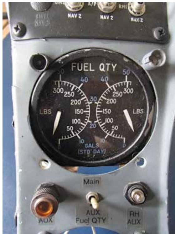
Figure 4 G-BXUY fuel quantity gauge (electrical power not applied)
