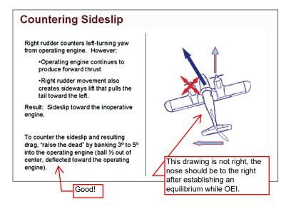
Sideslip is the angle at which the relative wind meets the longitudinal axis of the airplane. In all-engine flight with symmetrical power, zero sideslip occurs with the ball of the slip-skid indicator centered. Pilots know this concept as "coordinated flight." In OEI flight, however, zero sideslip occurs with the ball slightly out of center, deflected toward the operating engine.
