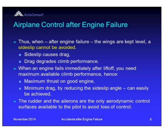
Thus, when – after engine failure – the wings are kept level, a sideslip cannot be avoided. However, ...
